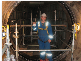
Testing 102" weld with only ½-gallon of water at 250 psig!
